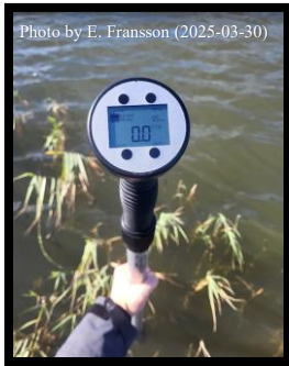
Figure 4 shows the velocity measurements obtained using the flow probe (Global Water FP111) in Göta Älv.
